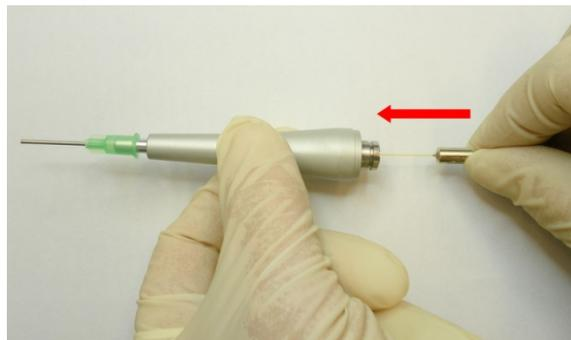
After this, place the handpiece front part centrally on the rear handpiece part. Then press both parts together in the handpiece longitudinal direction until the interlock ring can be heard to engage.
