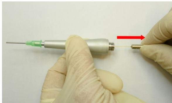
The fibers can be changed during operation with the device switched on. Fibers must not be replaced during laser emission under any circumstances!
