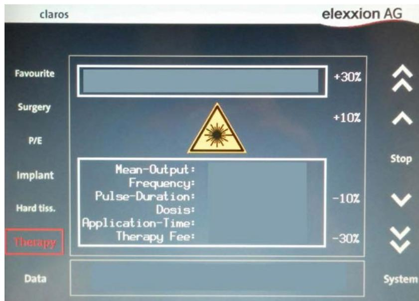
**Note:** From here on actuating the foot switch results in emission of laser radiation! The application name is shown in the upper frame. In the middle of the main windows, a flashing warning symbol appears during laser emission. An alert signal also sounds.
