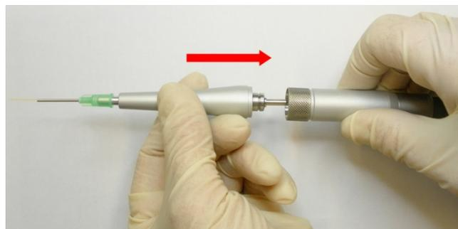
The fiber can be removed after use. (To do so, ensure that the soft metal tip has been bent straight again or removed beforehand.)
