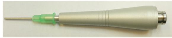
Push application fibers carefully into the handpiece front part from behind as far they will go. (Caution: glass fibers can break)
