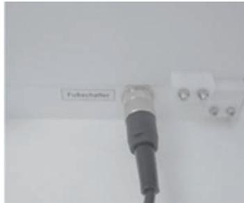
3. Insert the interlock plug into the "Interlock" connection socket behind the side housing cover and secure it by turning the union nut clockwise.
